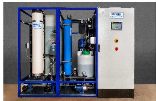
Chemical enhanced cleanings with the addition of alkaline and acidic surfactant-containing membrane cleaners take place automatically with the integrated CIP module.
